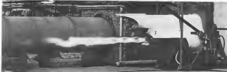
At full thrust the Spectre will jet fuel which combusts with the oxygen released by the HTP and boosts the combustion temperatures to 6,000 F and the thrust to 4,000 lb.
